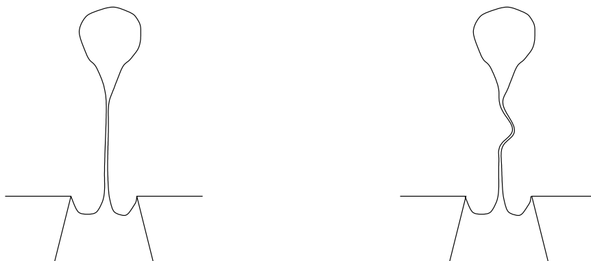
Figure 1: Schematic diagram of asymmetric break-off.
