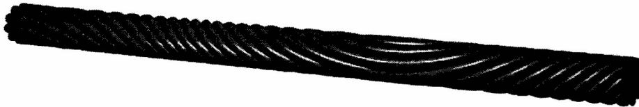
Figure 1: Schematic diagram of the loose tubes wrapping around the central strength member. The wrapping starts off helically in an anticlockwise direction, then reverses to wrap clockwise.
